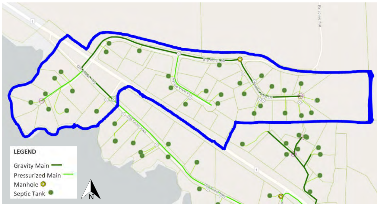
Figure 4.4.1-6 Lift Station 1 Shed Area (Outlined in blue)
